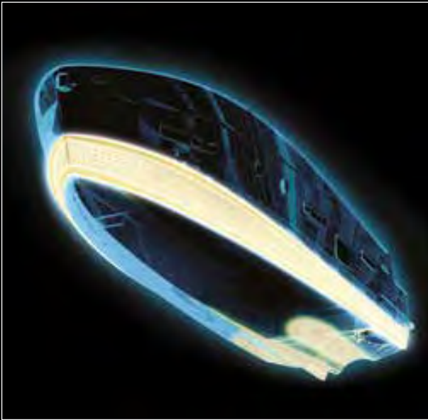
Dual Mode semi-planing hull with tunnel, skeg and vertical bow (Magellano Collection)
