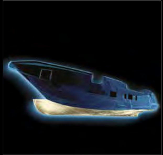
D2P (Displacement to Planing) hull with a double chine and wave piercer (reserved for several models in the Grande Collection)
